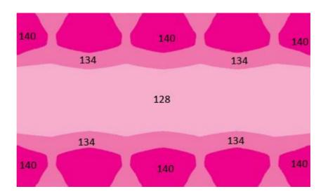
Average: 134 μMol/m²/s Maximum: 140 μMol/m²/s Minimum: 128 μMol/m²/s Uniformity: 92%
